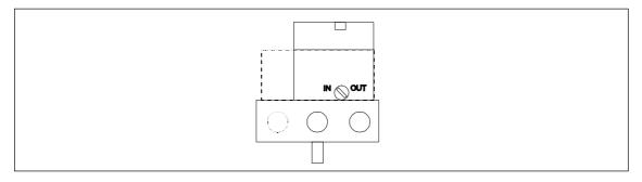
Figure 2-6 Purge air switch on the valve block, view of the positioner onto pneumatic connection side with cover open
