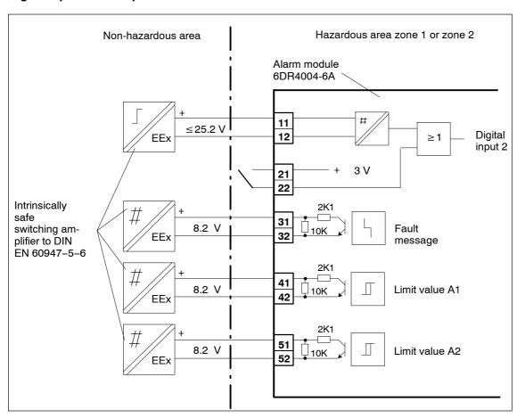
Figure 3-24 Alarm module 6DR4004-6A, EEx i
