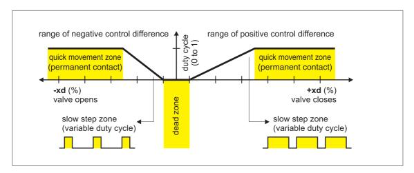
Figure 2-8 Method of operation five-point switch
