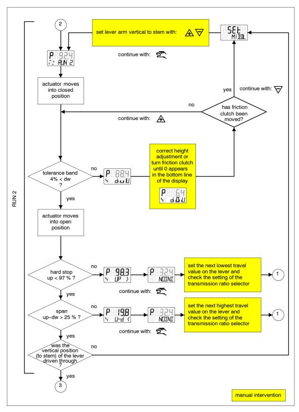
Figure 3-35 Automatic initialization part 2 (in linear actuators)
