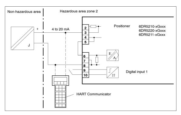
Figure 3-27 Two-wire connection, EEx n
