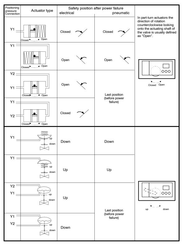
Figure 2-5 Pneumatic connection positioning
