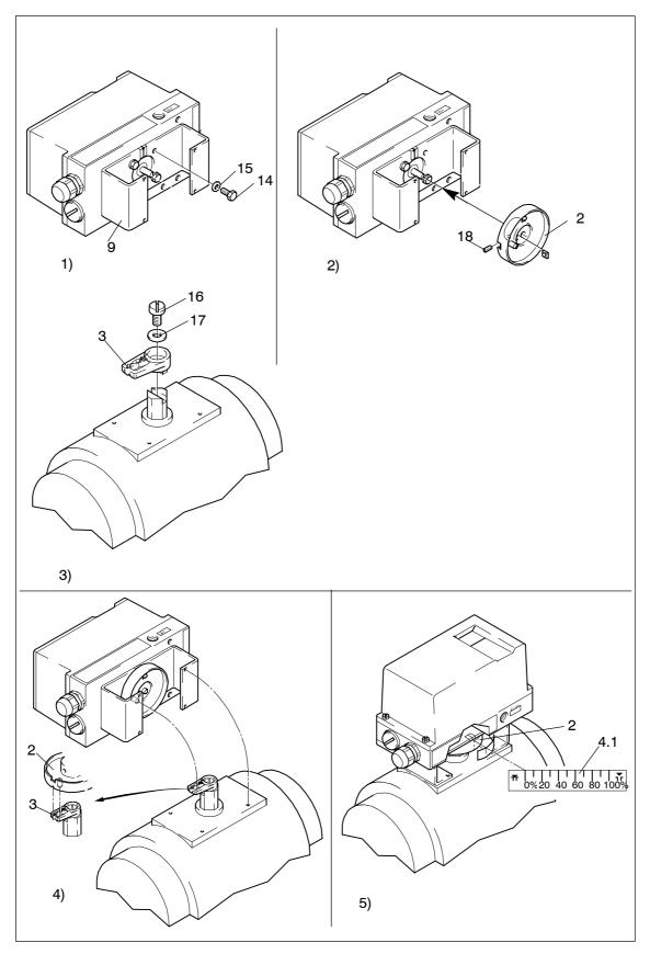
Figure 3-8 Assembly procedure (part-turn actuator)
