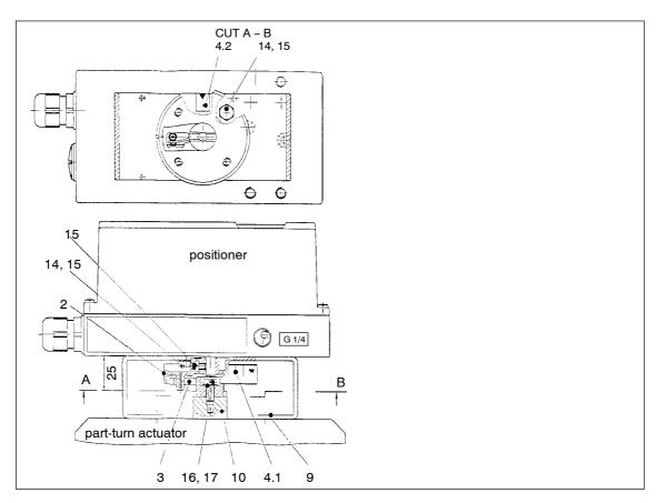
2 Coupling wheel 10 Feedback shaft 3 . Carrier Hexagon head screw M6 x 12 14 4 Multiple plate 15 Lock washer S6 Fillister head screw M6 x 12 4.1 Scale 16 4.2 Pointer mark 17 Washer VDI/VDE 3845-mounting bracket 18 Hexagon socket head screw
