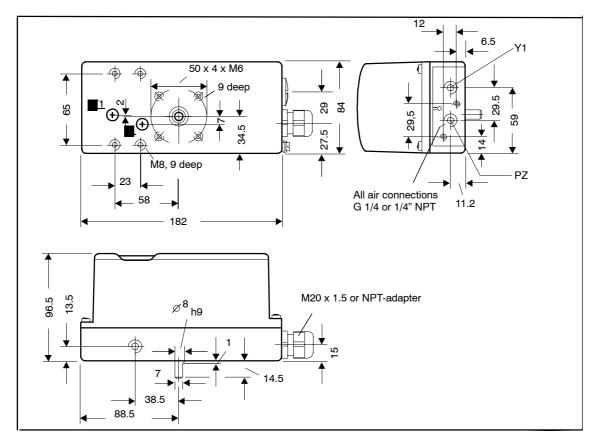
Figure 3-3 Dimensional drawing version metal housing 6DR5xx1
