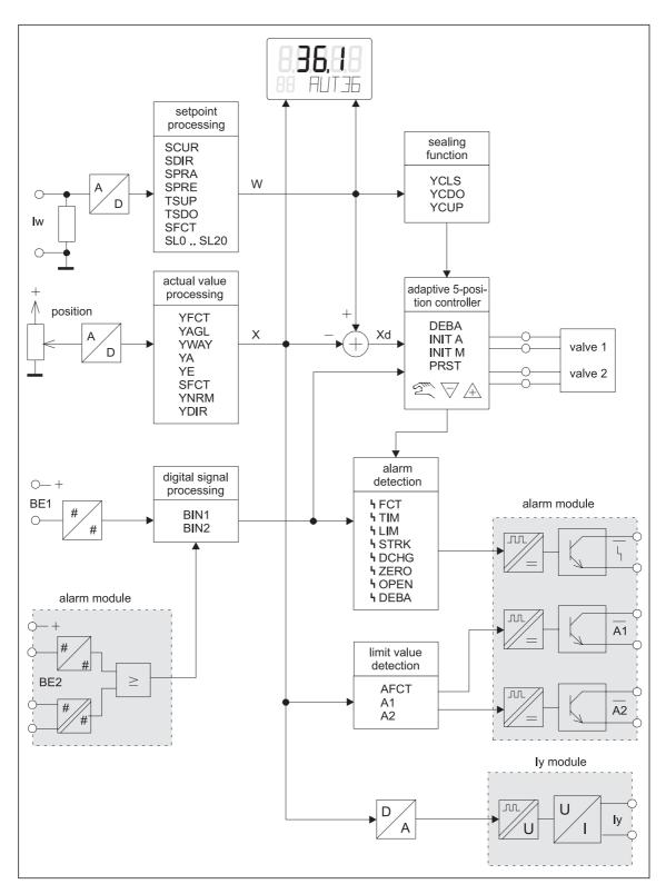
Figure 4-7 Configuration block diagram
