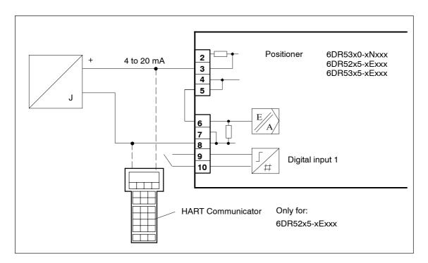
Figure 3-14 Two-wire connection
