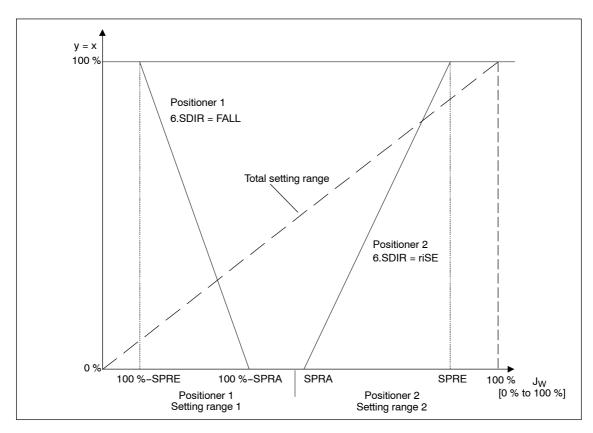
Figure 4-8 Example: Split range-operation with two positioners
