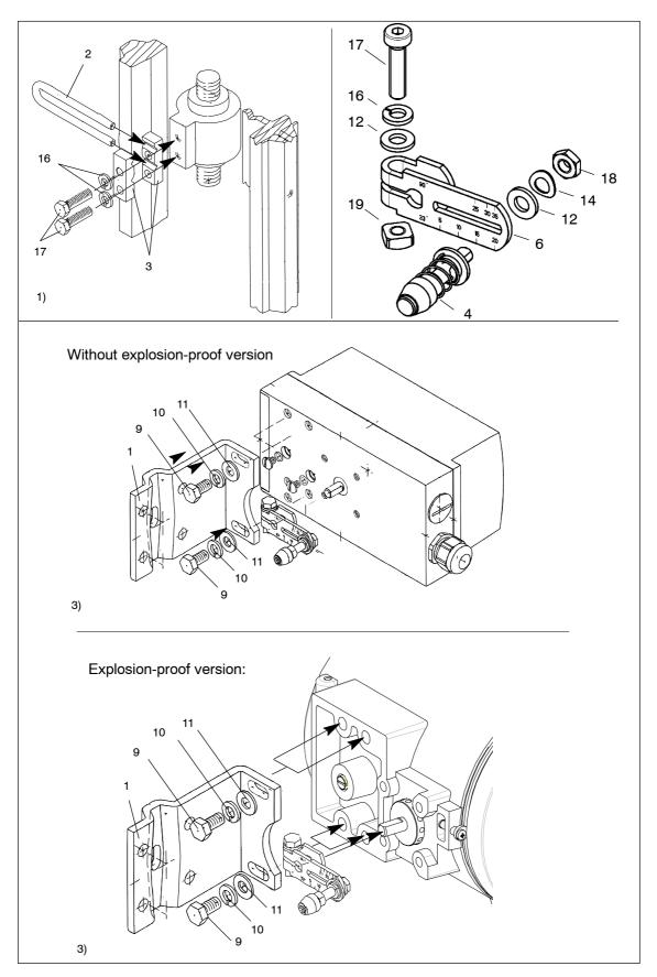
Figure 3-7 Assembly procedure (linear actuator)
