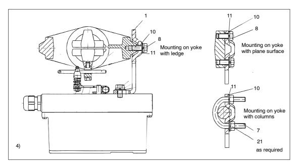
Figure 3-7 Assembly procedure (linear actuator) continued
