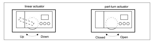
Figure 3-32 Direction of action of the actuators
