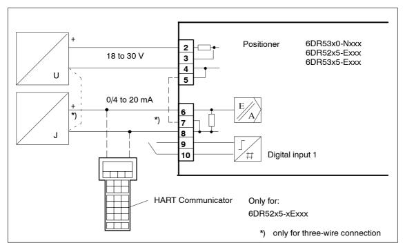
Figure 3-15 Three-/four-wire connection
