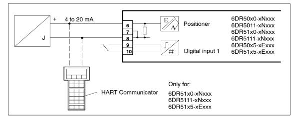
Figure 3-13 Two-wire connection
