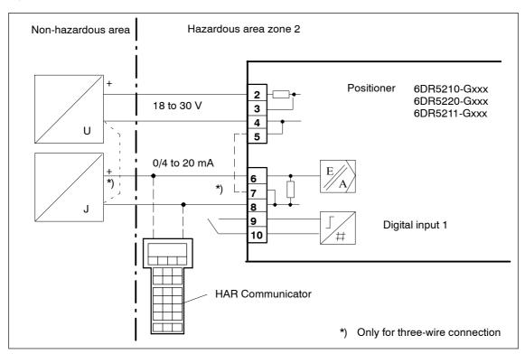
Figure 3-28 Three-/Four-wire connection, EEx n
