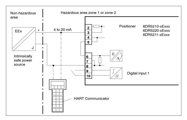
Figure 3-20 Two-wire connection, EEx i
