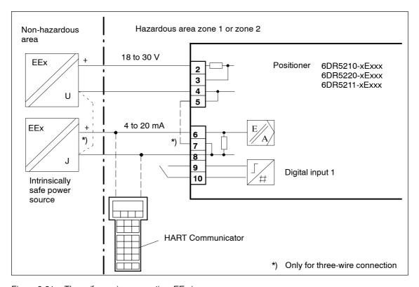
Figure 3-21 Three-/four-wire connection, EEx i
