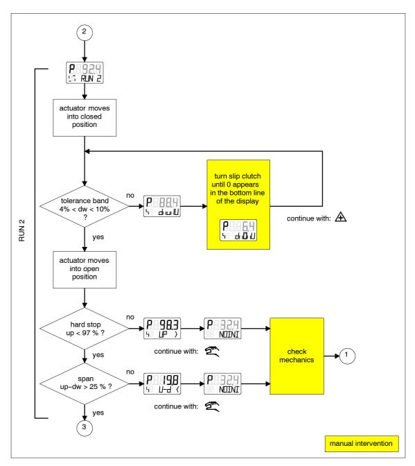
Figure 3-34 Automatic initialization part 2 (in part-turn actuators)
