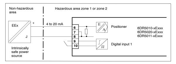
Figure 3-19 Two-wire connection, EEx i
