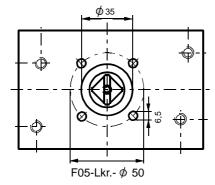
Figure 3-11 Attachment of part-turn actuator, mounting console (scope of delivery actuator manufacturer), dimensions
