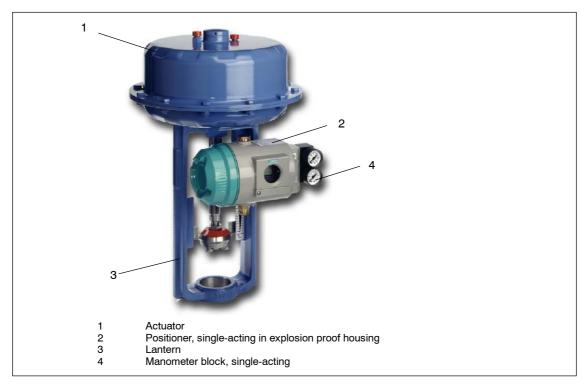
Figure 1-3 Explosion proof version of the positioner mounted on linear actuator (single-acting)
