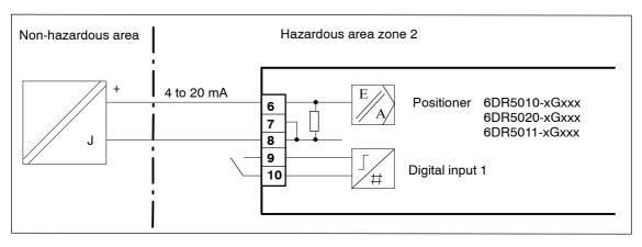
Figure 3-26 Two-wire connection, EEx n
